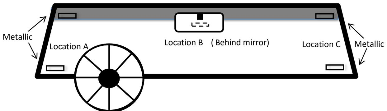
**HOWEVER**, if your vehicle has black dot shading (not solar tint), you may install transponder in the shaded area but at least 2" inches away from all metallic surfaces. Black shading are very small dots creating a shaded area at the top of most late model vehicle windshields. This is not a solar tint and is not solid throughout.
