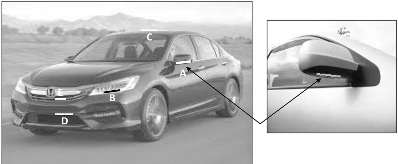
The images above show recommendations for the placement of transponders. Notice the horizontal parallel fitment as would be viewed from the RFID reader. The transponders do not need to be visible to the naked eye, only need to be visible to the radio signal as it can pass through most non-metallic materials. The letters above show five (5) ways the Q-500 transponder may be placed upon a vehicle. Placement (A) shows transponder installed underneath the driver side-view mirror.
